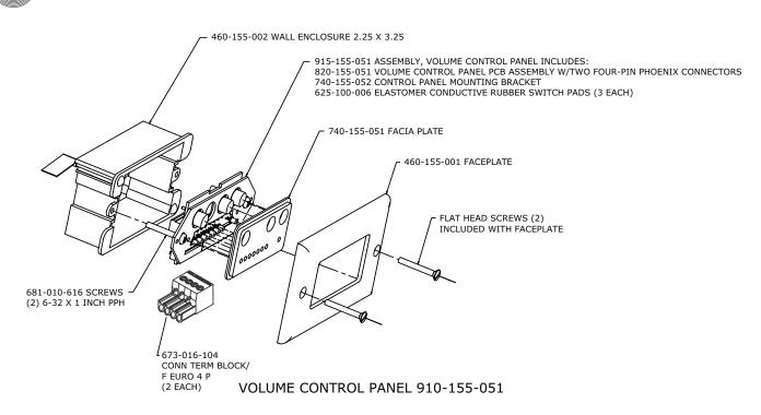
Figure C.6. Volume Control Panel Assembly
